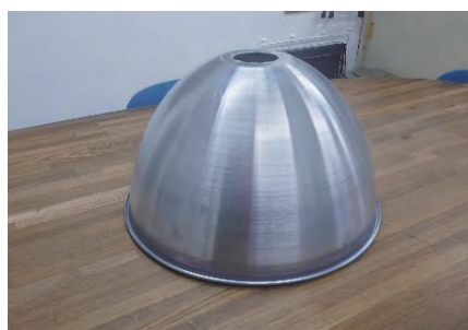
Spatula drawing processing sample (aluminum)
