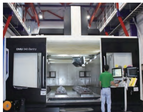
Machining center (DMG Mori Seiki 5-axis MC DMU340 Gantry)
