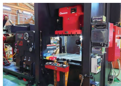
200ton digital electric servo press
