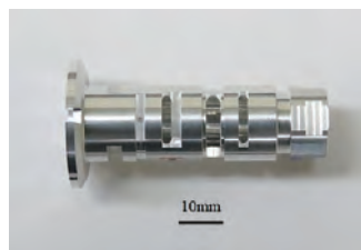
Industrial machinery parts (A5056)
