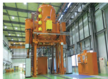
Vertical single-chamber vacuum furnace ( \phi 2100 \times H2700 )
