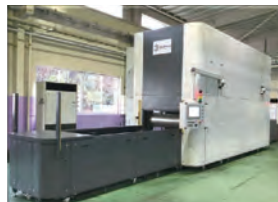
Hydroforming machine(Quintus) 2000X1000XH120
